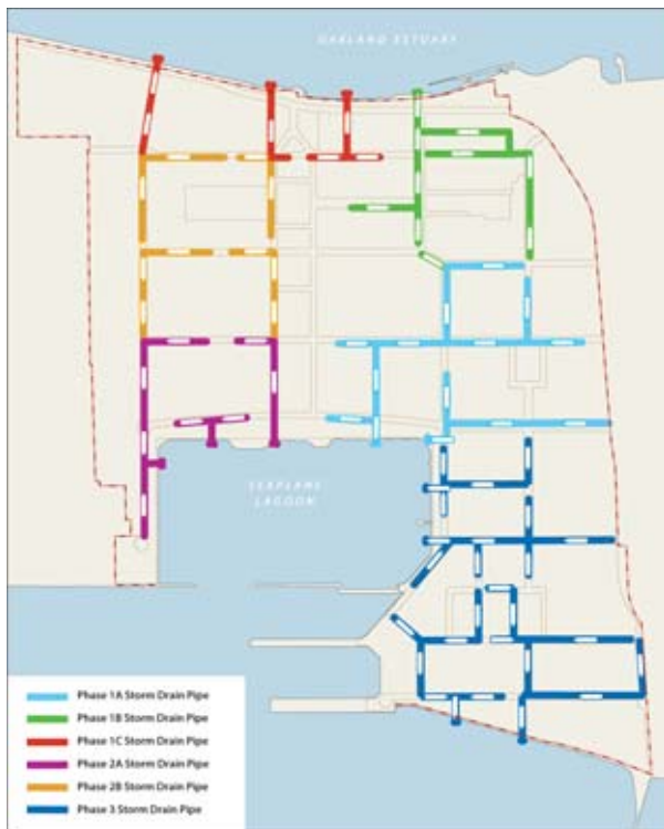
FIGURE 17: STORM WATER SYSTEM
